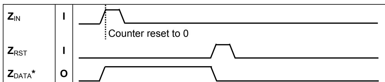
\*Note:  $Z_{DATA}$  will be Hi-Z (tristate) unless CS is low. Pull CS low to read the data.
