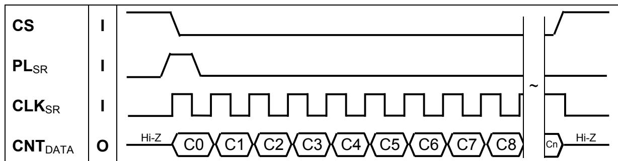
C0 is the LSB of the count value, increasing to Cn (n - number of counter bits).
