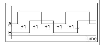
The decoder samples the filtered  $A_1$  and  $B_1$  signals ( $A_2$  and  $B_2$  for channel 2), and calculates the up/down transition based on current and past state. When a transition is detected, either CNT1<sub>UP</sub> or CNT1<sub>DN</sub> will go high for one clock cycle (CNT2<sub>UP</sub> or CNT2<sub>DN</sub> for channel 2). These pulses also form inputs to the internal counter.
